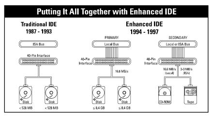
Enhanced IDE (Enhanced Integrated Drive Electronics) is the latest standard used to handle communication between hard drives and the central processing unit. As with its predecessor, Enhanced IDE consists of interface controller electronics that reside on the hard drive, along with some important new features required to keep pace with the continually evolving computer industry.
