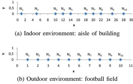
Fig. 3. Topology layout of the 10 sensor nodes in indoor and outdoor environments. Nodes  $N_2 \dots N_{10}$  belong either to the *connected*, *transitional* or *disconnected* region of  $N_1$ , so that links  $(N_1 \leftarrow N_i)$ , for  $i \in [2, 10]$ , have different qualities.
