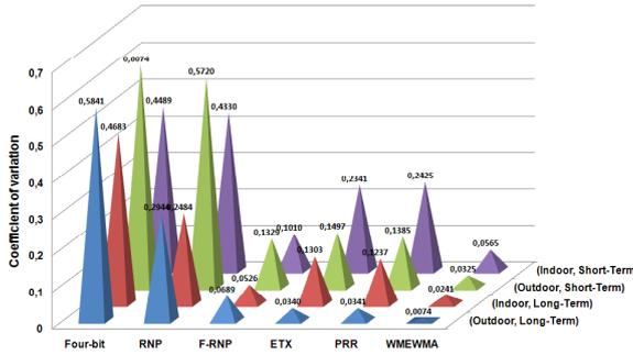
Fig. 8. Stability of link quality estimators (Traffic Pattern 2)
