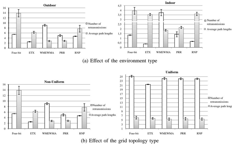
Fig. 13. Performance comparison in terms of number of retransmissions and average path length
