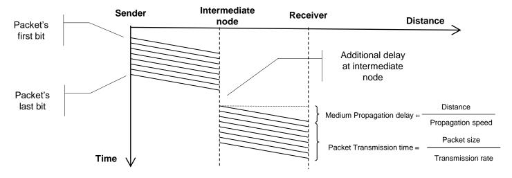
As we can see on the image above, the latency added by an intermediate node equals the **packet transmission time**. However, intermediate nodes may not be able to send the packet as soon as it's received, this introduces an **additional delay**. Intermediate nodes use queues (FIFO) to store received packets before emitting them, these queues operate as buffers and are essential because the intermediate node may not be able to emit packets at the same rate they are being received.
