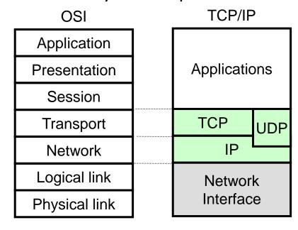
The TCP/IP stack consists of several protocols in addition to the IP, the most importants are **UDP** (**User Datagram Protocol**) and **TCP** (**Transmission Control Protocol**). UDP – **connectionless** packet protocol without reliability, only simple error detection. TCP – **connection-oriented** reliable protocol with sliding window flow and error control. Of these two, the most widely used over the Internet is TCP.
