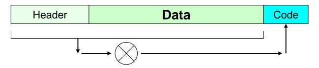
The sender uses the function to calculate the code, and then, adds it to the packet. In some cases, the code is added to the packet header, but in can also be added to the tail as presented on the image above.
