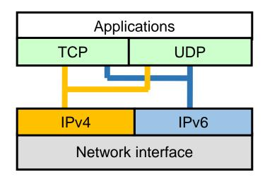
As we can notice in the figure above, in each layer, there are frequently several protocols running. This is possible thanks to tag-based multiplexing. Tagging ensures data from a layer implementation X in one node, ends up being delivered to the same layer implementation X on the destination node.
