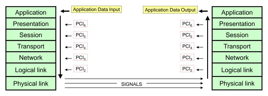
The exchange of information via each layer's PCI is related to that layer's specific features and follows a set of rules known as protocol. Thus, each layer has its own protocol.
