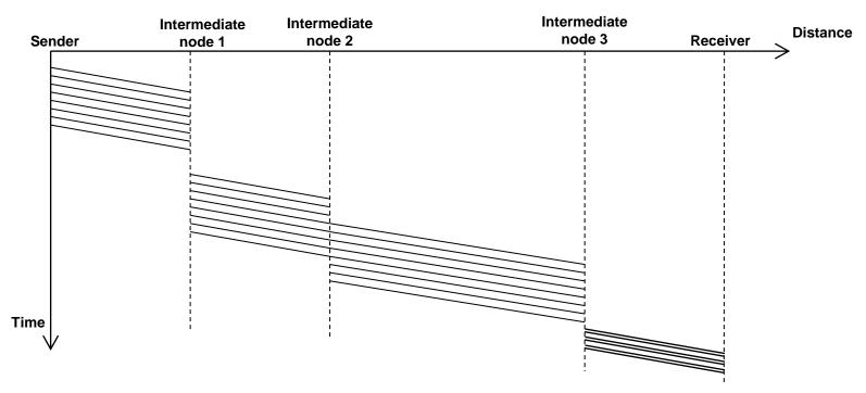
Intermediate nodes 1 and 3 fully receive packets before starting to emit them, this is called **store & forward**. Some types of networks allow, however, another operation mode called **cut-through**, that is the case of intermediate node 2. Another factor to take account for is that intermediate nodes may receive and send at different data rates, that is the case of intermediate node 3.
