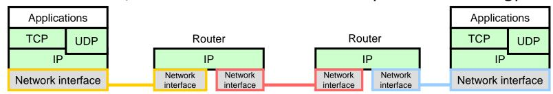
The diagram above represents three different layer two technologies being used: yellow, red, and blue. By using IP, a node connected to the yellow LAN is able to communicate with a node connected to the blue LAN.
