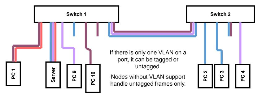
Port-based VLANs are the most often used, but some switches also support MAC address based VLANs, where the VLAN to which a node belongs is determined by the node's MAC address.
