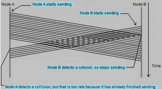
To ensure collision detection by all nodes, there's a **minimum packet size** of 64 bytes (this sets a minimum transmission time), also there is a **maximum segment size** (sets the maximum propagation delay). These two limits guarantee a collision at any point is detected by the farthermost node before the packet is completely transmitted. This is called the **collision domain**.
