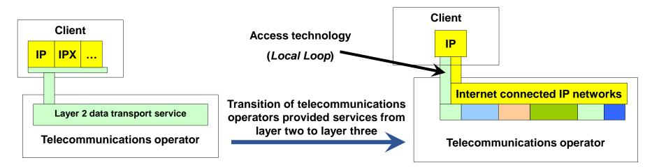
A layer two technology is still required to transport IP packets between the costumer and the operator. This connection is known as **Local Loop**. The local loop can be based on a new wiring installation, typically optical fibre, but that's always an expensive option. There are other solutions:
