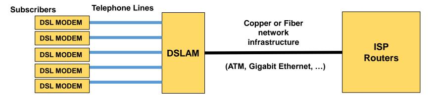
Each subscriber's traffic is sent separately over the network infrastructure by using different virtual channels (ATM) or different VLANs (Ethernet).
