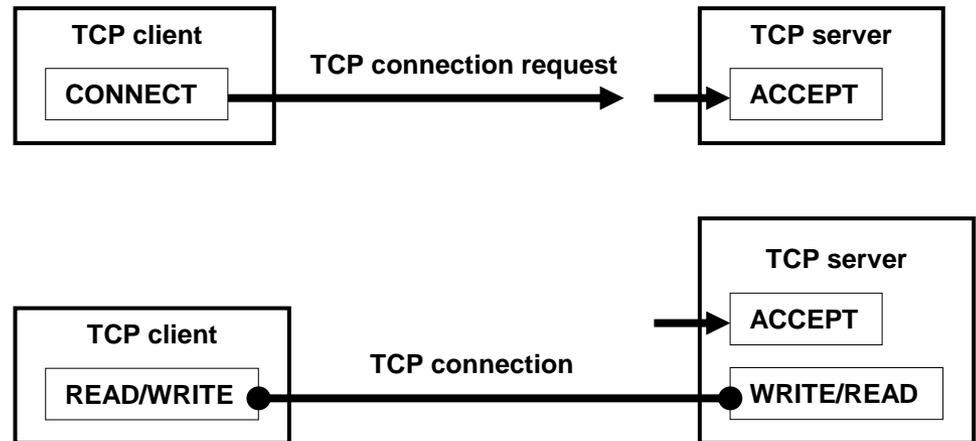
The application protocol defines the sequence of messages, and messages contents to be exchanged between the client and server over the TCP connection. Because it's a permanent and dedicated channel, the TCP connection allows a session of successive interactions, not just a single request and a single reply like with a typical UDP client-server.
