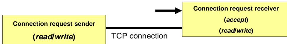
On the receiver side, the acceptance of the connection (accept) has created a new socket associated to the TCP connection, yet the original socket remains open to receive other connection requests.
