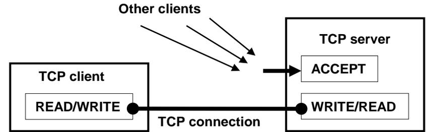
Thus, it must handle with two sockets, keeps accepting new clients on the initial socket, and exchanges information (requests and replies) with the connected client through the new socket.
