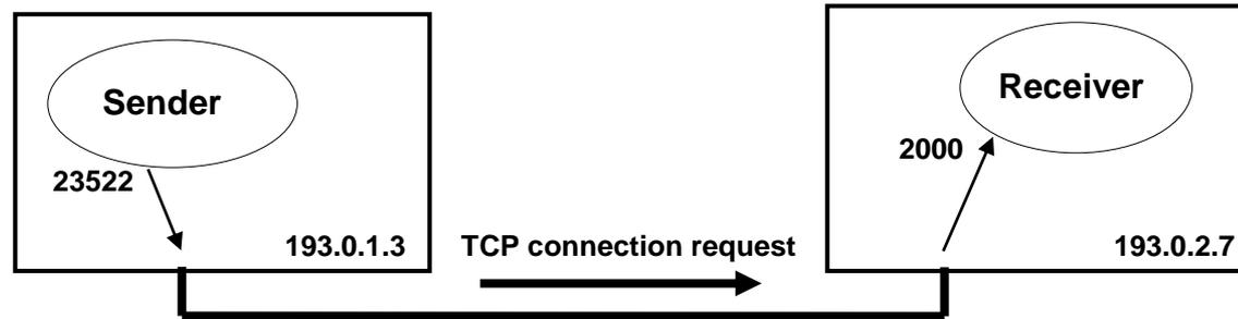
After the TCP connection establishment, each connected socket will also have associated with the remote IP node address and the remote port number.
