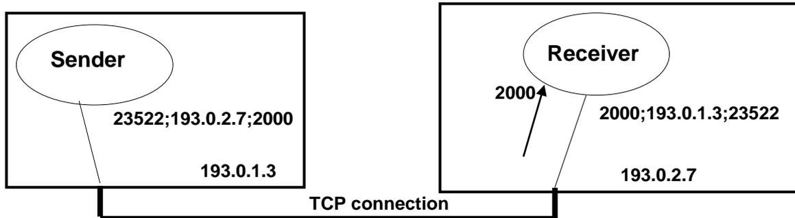
The receiver has now two sockets associated to the same local port number. Even though only the connected socket has a remote address associated.
