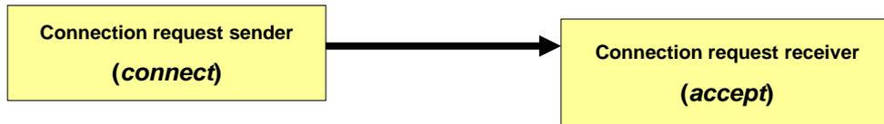
The sender application triggers a connection establishment request (connect) to the IP address of the receiving node and port number used by the receiving application.
