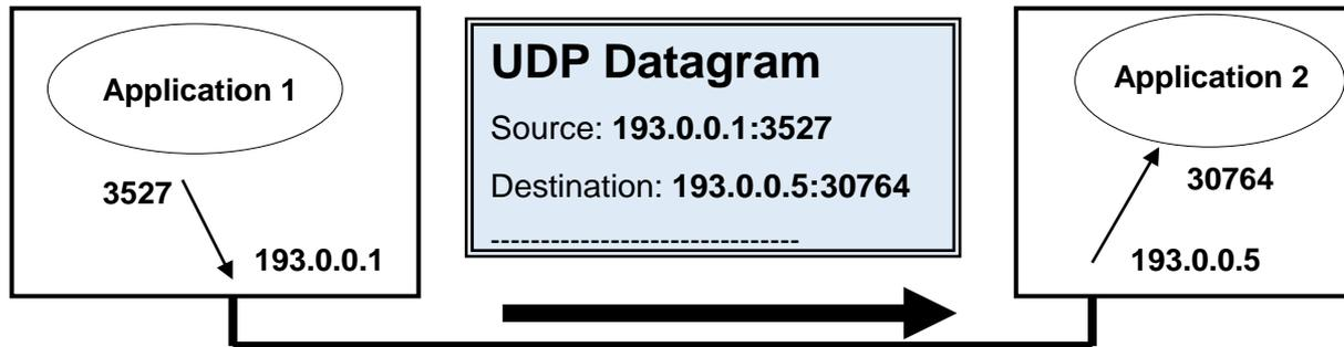
Associating a local port number to an application is often called binding. This is something applications must request to the local operating system. One thing the operating system will ensure is that there's only one application using each port number.
