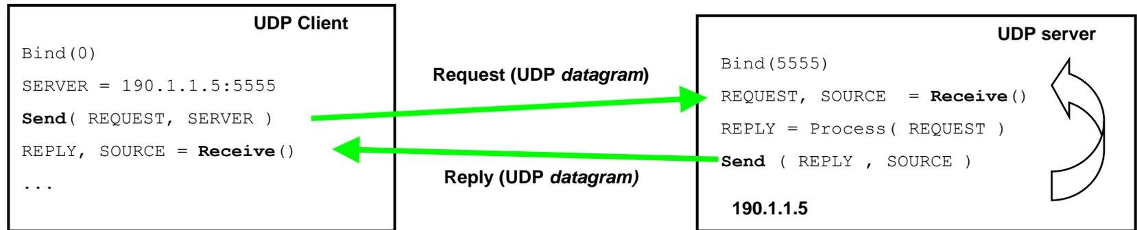
In this case, problems with UDP lack of reliability will arise on the client side. The issue is, the client trusts there will be a reply from the server, if no reply is received the client blocks forever waiting for a reply that will never arrive.
