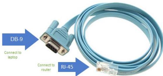
Figure 3 - RJ45 to DB-9 roll-over console cable
