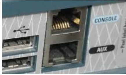
Figure 2 - The console port of a Cisco 2811 router
