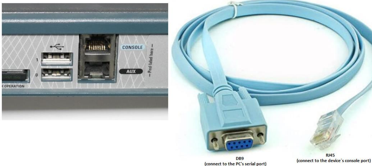
Figure 1 – The console port in a 2811 Cisco router and a roll-over cable
