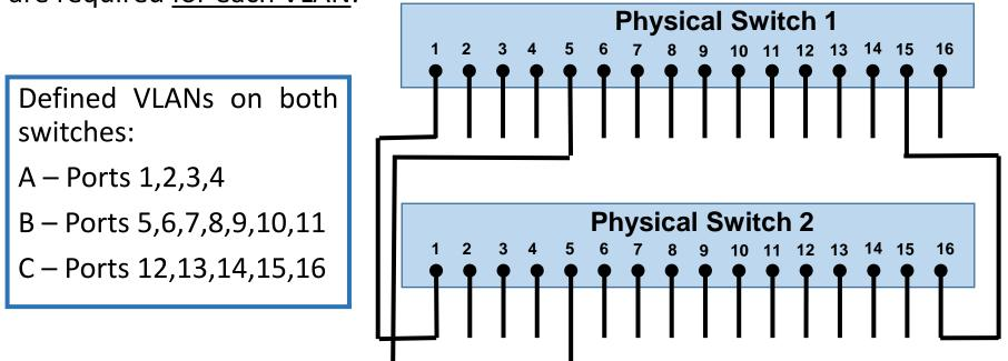
Current switches allow a workaround to save a lot of hardware (ports and cables), it's called **VLAN frame tagging**. Such switches are capable of assigning one same port to more than one VLAN.
