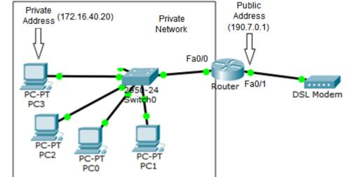
Static NAT is most useful for providing access from the internet to servers connected to a private network. In the above configuration, we can see that any access from the internet to address 190.7.0.1 is going to be redirected (DNAT) to the private node 172.16.40.20.
