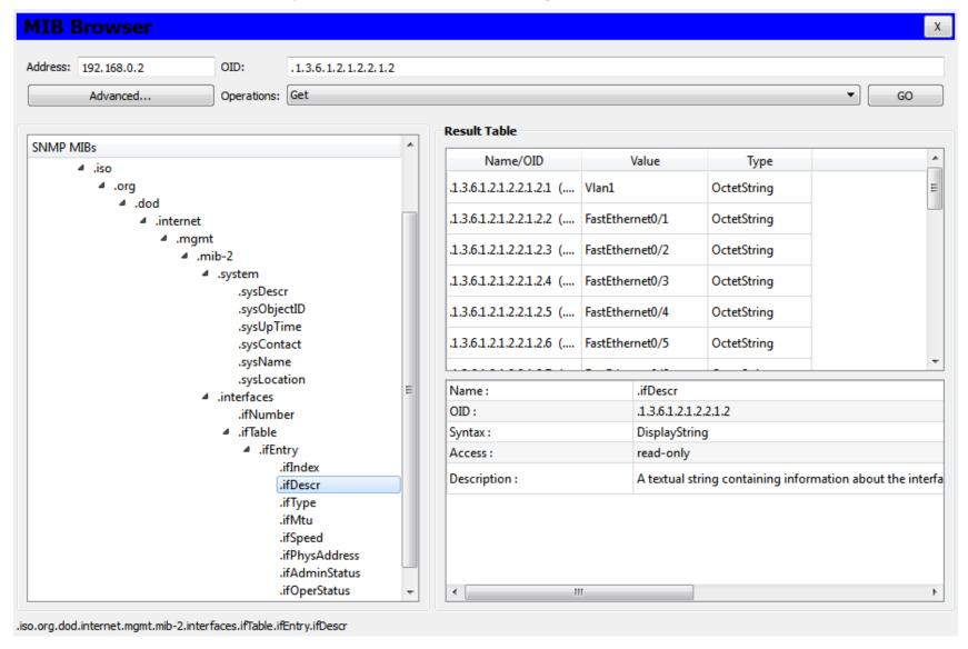
On a real device MIB, each entry in an interfaces table has several other objects, not present in Packet Tracer devices:
