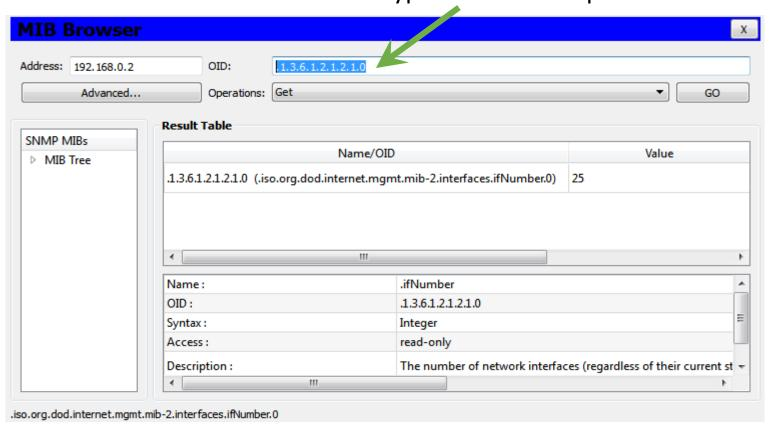
We got 25 interfaces for this switch; they are 24 physical interfaces and the VLAN interface we have created to establish the switch IPv4 address.
