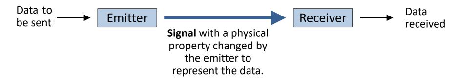
By changing signal properties like intensity, frequency or phase, data to be sent is represented.
