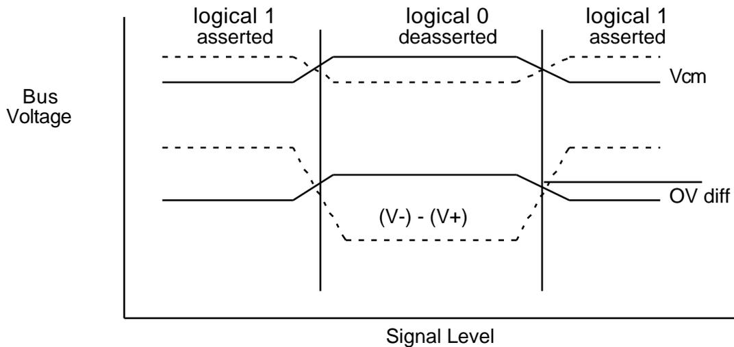
**Fig. 3: LVD Signal polarities**
