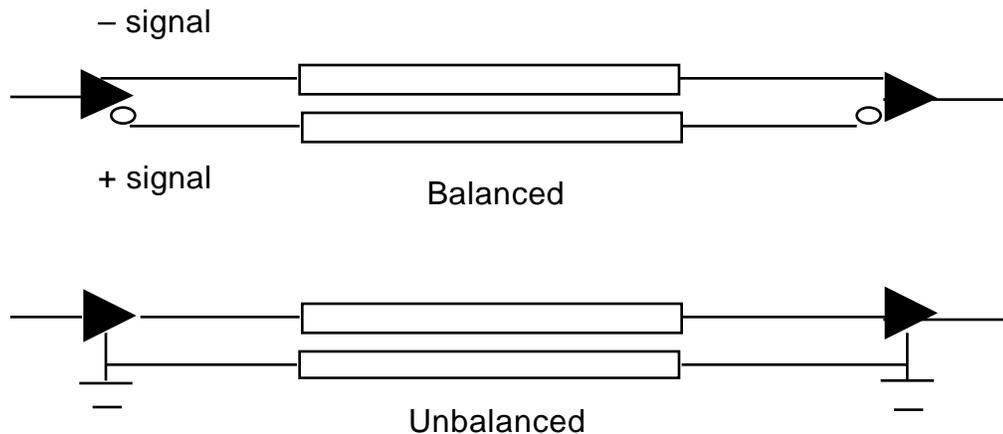
**Figure 1: Balanced vs unbalanced transmission**
