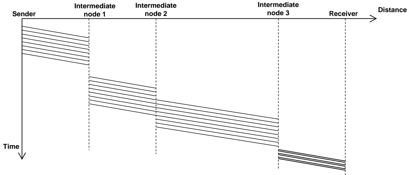
Intermediate nodes 1 and 3 fully receive packets before starting to emit them, this is called **store & forward**. Some types of networks allow, however, another operation mode called **cut-through**, that is the case of intermediate node 2. Another factor to take account for is intermediate nodes may receive and send at different data rates, that is the case of intermediate node 3.
