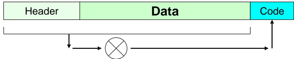
The sender uses the function to calculate the code, and then, adds it to the packet. In some cases, the code is added to the packet header, but it can also be added to the tail as presented on the image above.
