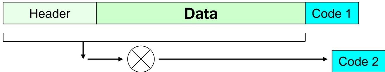
At the image above, **Code 1** was calculated by the sender and **Code 2** by the receiver.
