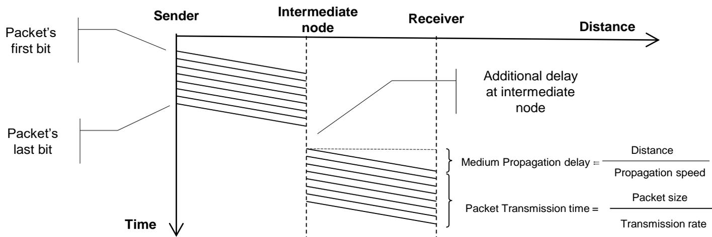
As we can see on the image above, the latency added by an intermediate node equals the **packet transmission time**. However, intermediate nodes may not be able to send the packet as soon as it's received, this introduces an **additional delay**. Intermediate nodes use queues (FIFO) to store received packets before emitting them, these queues operate as buffers and are required because the intermediate node may not be able to emit packets at the same rate they are being received.
