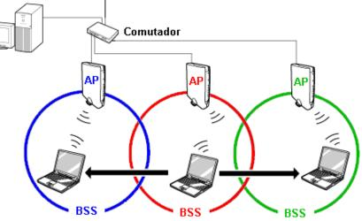
By using the same SSID on all cells, all cell will be part of the same ESS. Wireless network nodes can then move freely between cells of the same ESS without losing network access. The transparent transfer from cell to cell is known as **roaming**.
