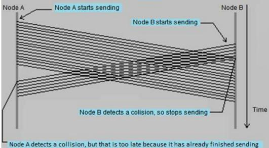
To ensure collision detection by all nodes there's **minimum packet size** of 64 bytes (this sets a minimum transmission time), and there is a **maximum segment size** (sets the maximum propagation delay). The segment size limit guarantees a collision at any point is detected by the farthermost node before the packet is completely transmitted. This is called the **collision domain**.
