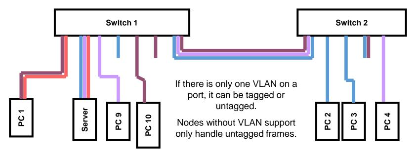
Port-based VLANs are most often used, but some switches also support MAC address based VLANs, where the VLAN to which a node belongs is determined by the node's MAC address.
