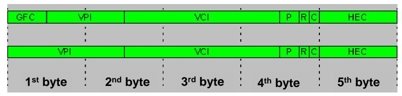
In UNI cells (top) VPI is zero, VPI is defined only in cells traveling inside the network. The GFC field (Generic Flow Control) only exists in UNI cells, it's used for local flow control and multiplexing.
