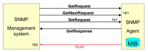
The **Request ID** field identifies a specific request, the value will be copied to the reply relating one with the other. Because SNMPv1 uses a unreliable transport (UDP) establishing this relation is important.
