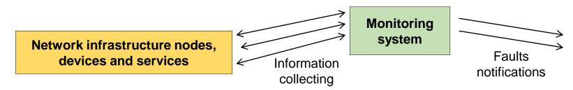
The main activity for a monitoring system is information collecting, this is most often accomplished through **active checks**. With active checks, for each item to be checked, the monitoring system will periodically take an action to retrieve its status.
