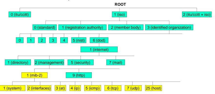
Each object class is identified by following the numbers sequence starting on root until the branch is reached, for instance **internet** object is identified by the **1.3.6.1** OID, all objects in sub branches will be started by that OID. Objects related to network management are started by **1.3.6.1.2.1**, highlighted in yellow.
