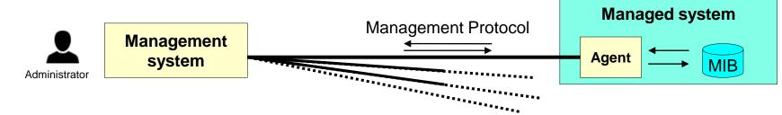
The **management system** is the central control point from where requests are sent to **managed systems**. A **management protocol** is used for these client-server dialogs.
