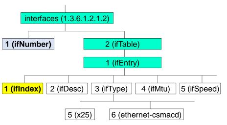
SNMP uses OIDs, however an OID refers to an object class, not an instance. And of course, there can be several instances of the same class. SNMP adds one more number to identify instances starting by zero. To get the number of interfaces in a network device the request must be for the first instance of **ifNumber** class: **GET 1.3.6.1.2.1.2.1.0**
