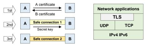
Many application protocols use the TLS layer instead the TCP layer to create safe versions of themselves, for instance HTTP runs over TCP, HTTPS is the same protocol running over TLS.
