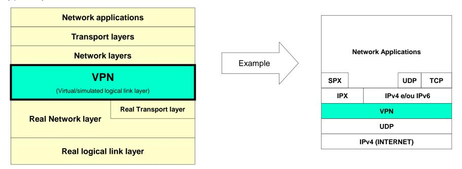
**Virtual** stand for it not being a real physical infrastructure, its just a point-to-point tunnel created over an already existing network. Because information sent through the tunnel is encrypted it is also called **private**. Even though every VPN uses the same principles, they can be classified into types with several criterions.
