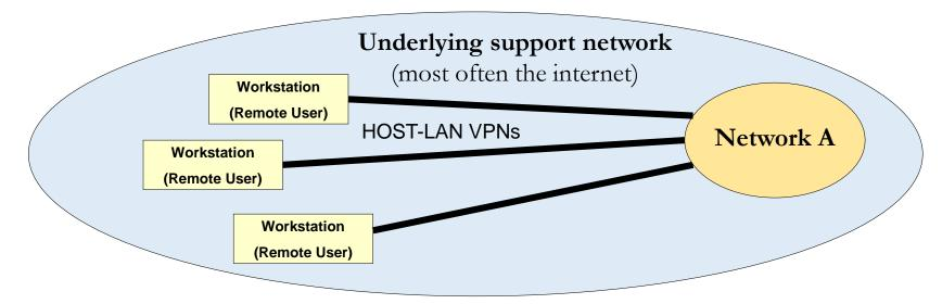
Users authentication and access control are enforced by the VPN server. Once the access is granted, the user's workstation is provided with an IP address belonging to the remote network. The workstation operates as if it was directly connected to that network, this allows the VPN client to bypass firewalls around the remote network and also guarantees privacy on transactions with the network.
