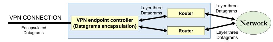
Because endpoints are routers, broadcast traffic is not forwarded. For a layer three VPN, routeing configuration is required because its not a single network anymore.
