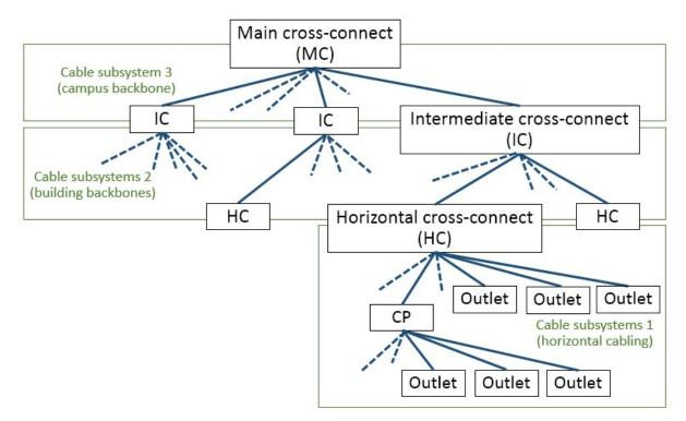
The campus backbone makes sense when there are several buildings to be covered, for each building we will then have an intermediate cross-connect (IC).
