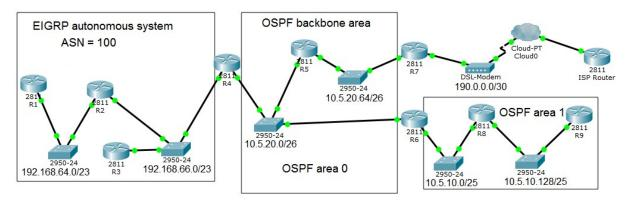
IPv4 network addresses are presented at the image, below layer two devices.
