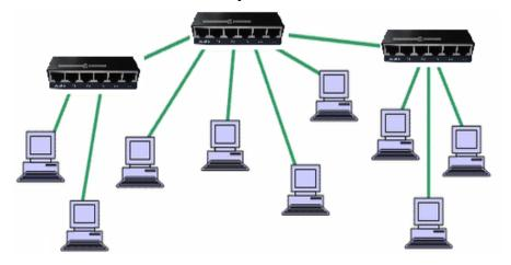
Although having a star topology, it's a shared medium network, from many points of view equivalent to a bus topology. At layer 2 a medium access control (MAC) protocol must in enforced, otherwise collisions will occur when two nodes emit a signal at the same time. A collision means two or more signals are mixed on the transmission medium and all data is lost.
