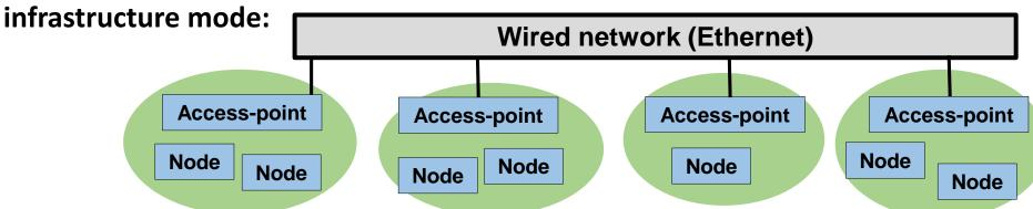
An access point, also know as base-station, is a layer two active device, first of all, it operates as a frame switch, retransmitting frames. Because each access point has a wired connection (Ethernet) it will not only retransmit frames between wireless nodes but also between wired nodes (Ethernet) and wireless nodes.
