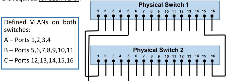
Current switches allow a workaround to save a lot of hardware (ports and cables), its called **VLAN frame tagging**. These switches are capable of assigning the same port to more than one VLAN.
