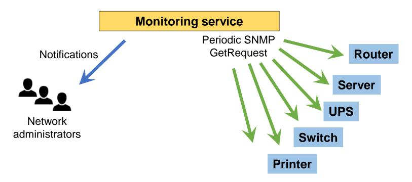
The **monitoring service** runs in background with the mission of **periodically checking** if all components are conforming to pre settled requirements, if a deviation is detected, **network administrators are notified**.
