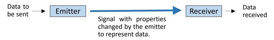
The **receiver** listens for the signal, measures the properties the **emitter** is changing, and thus, gets the originally sent data.
