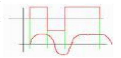
Both attenuation and propagation delay depend on frequency, so whenever a non-sinusoidal signal is sent, the received signal will be rather distorted. To overcome this problem, emitters apply a passband filter to transform the non-sinusoidal signal into a fairly sinusoidal signal before sending it.
