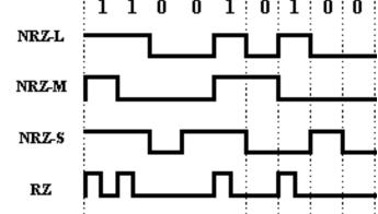
In NRZ-M each one symbol is represented by a level transition, contrariwise for NRZ-S, each zero symbol is represented by a level transition.
