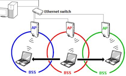
By using the same SSID on all cells, all cells will be part of the same ESS. Wireless network nodes can then move freely between cells of the same ESS without losing network access. The transparent transfer of a wireless node from one cell to another cell within the same ESS is known as **roaming**.
