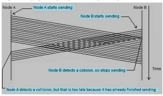
To ensure collision detection by all nodes, there's a **minimum packet size** of 64 bytes (this sets a minimum transmission time), also there is a **maximum segment size** (sets the maximum propagation delay). These two limits guarantee a collision at any point is detected by the farthermost node before the packet is completely transmitted. This is called the **collision domain**.
