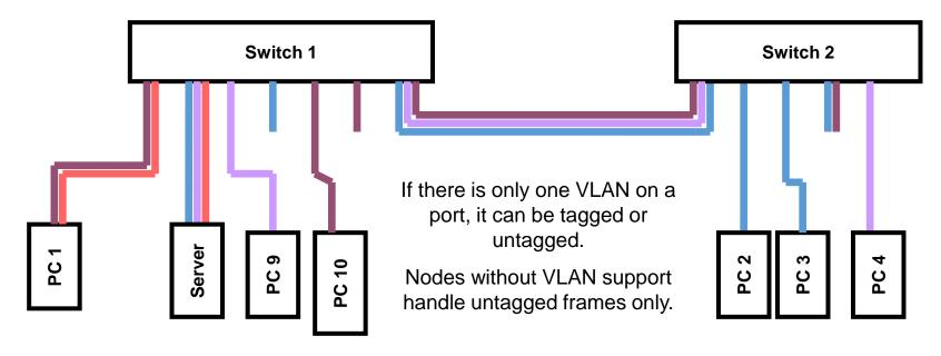
Port-based VLANs are the most often used, but some switches also support MAC address based VLANs, where the VLAN to which a node belongs is determined by the node's MAC address.
