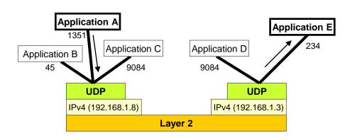
UDP application A is sending a UDP datagram to application E, to do so, it must specify not only the IPv4 node address application E is running on (192.168.1.3), but also the port number application E is using (destination port = 234).
