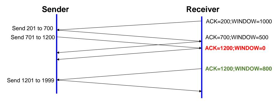
On the image above, the receiver initially reports a 1000 bytes window size, thus the sender is allowed to send up to more 1000 bytes. After two more 500 bytes segments, the window is exhausted (WINDOW=0), and therefore the sender is forbidden of sending more data. Later the receiver is ready for more 800 bytes of data and informs the sender with a segment containing WINDOW=800.
