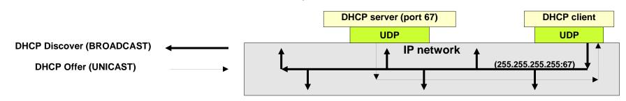
Once a **DHCP Discover** is received by a DHCP server, it will send back a **DHCP Offer** reply. The client may then select one of the received offers and request configuration data to that specific server. Configuration data provided to the client includes a unique available IPv4 address, the server keeps track of which IPv4 address it has assigned to each client by registering each client's layer two MAC address.
