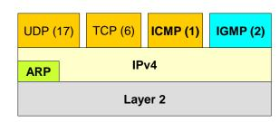
When a router receives an IPv4 packet with a multicast destination address (multicast group), it must know if there are nodes in other networks that belong to that multicast group, only if so, then the packet is required to be transmitted to those networks, otherwise it's pointless.
