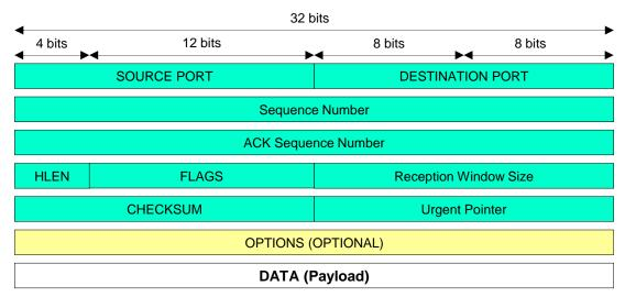
In a TCP data flow over a TCP connection, each byte has a sequence number. In the segment header, **Sequence Number** is the 32-bits sequence number of the first byte of data present in the segment payload. **ACK Sequence Number** is the 32-bits sequence number of the next byte the emitting node is expecting to receive from the counterpart, this implicitly acknowledges the good reception of all bytes sent before.
