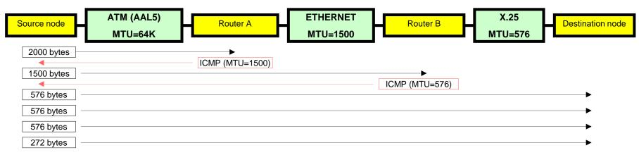
In the image above we can see that, after two errors, the sender finally sets the **path MTU** to 576 bytes, following communications to that destination node will always use packets smaller than 576 bytes. Of course, the path can change and may include a smaller MTU, then another correction will be required.
