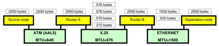
At first glance fragmentation is the ideal solution because it always takes the best advantage from each available MTU. In practice however, fragmentation causes delays on routers that must wait for fragments and reassemble packets.
