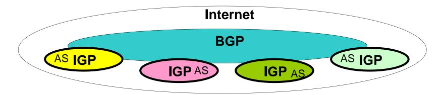
Each autonomous system has a unique ASN and some settled addresses blocks. Within the autonomous system, routing within the assigned address blocks is administratively autonomous and IGPs can be used for that purpose. Actually, BGP itself can also be used internally in a local AS but with private ASNs and not connected to the exterior BGP.
