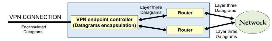
Because endpoints are routers, broadcast traffic is not forwarded. For a layer three VPN, routing configuration is required because it's not a single network any longer.
