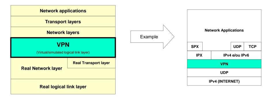
**Virtual** stand for not being a real physical infrastructure, instead it's a **point-to-point tunnel** created over an already existing network. Because information sent through the tunnel is encrypted, it's also named as **private**. Even though every VPN uses the same principles, they can be classified into types by following different criteria.
