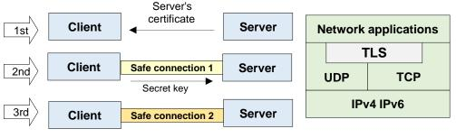
Finally, communications are encrypted by using by using the symmetrical key cypher.
