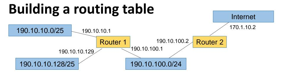
In this layout we have two routers and three local networks, Router 2 has an internet connection, near each router connection the router's IPv4 address is shown in the diagram.
