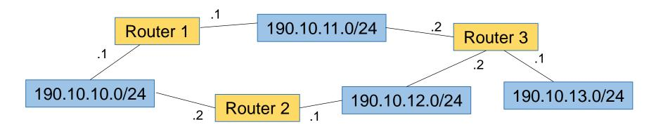
Before RIP starts to broadcast information about known networks, each router already knows the networks it's directly connected to, so routing tables are:
