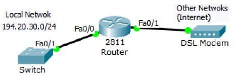
The first concern is: in which interfaces the access lists should be enforced. We could block external spoofing on Fa0/1 incoming traffic, or on Fa0/0 outgoing traffic. We could block internal spoofing on Fa0/0 incoming traffic, or on Fa0/1 outgoing traffic.
