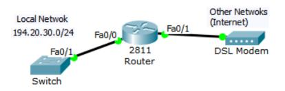
Access list 10 says any traffic with source address belonging to the local network should be blocked and all others should pass.
