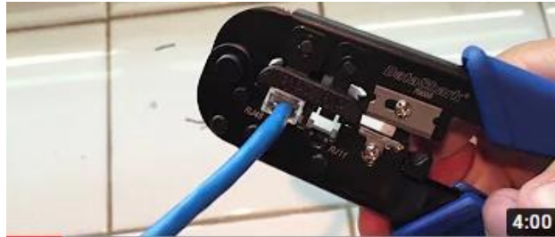
Figure 13 - Mounting a copper patch cord
