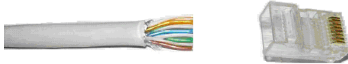
Figure 12 - UTP cable ready to be inserted into an RJ45 connector
