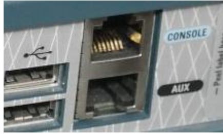
Figure 2 - The console port of a Cisco 2811 router
