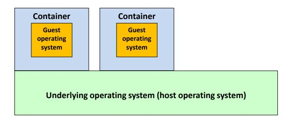
The container makes use of direct system-calls to the underling operating system, but is able to use resources only within the container.
