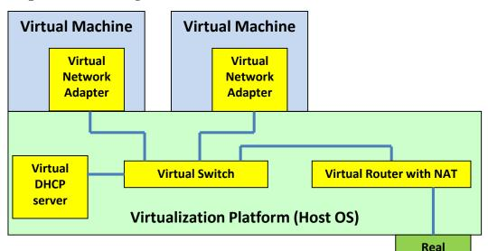
NAT stands for Network Address Translation, it allows the hiding of whole set of IP addresses belonging to a private network behind a single public IP address, in this case the public address of the real interface in the real network.
