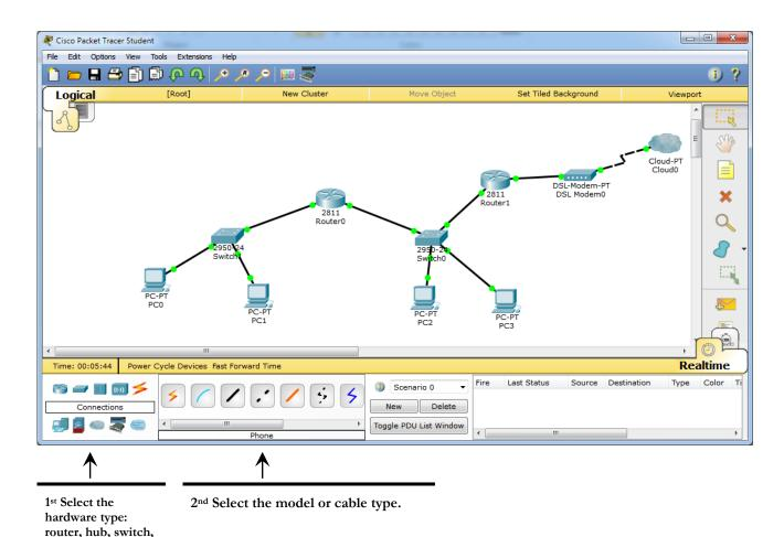
Once devices are connected and configured, Packet Tracer may be run in either real-time or simulation mode. In simulation mode the user is are able to see and follow, step by step, individual packets traveling around the created layout.
