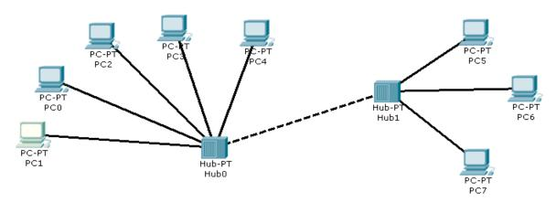
Notice: on Packet Tracer devices, copper ports are not auto MDI-X. Therefore, to connect two intermediate devices a cross-over cable is required.
