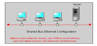
Even if collisions could be avoided the medium will never be totally available to a node as it may be busy with another node's signal. The effective sending data rate available to a node is, therefore, the medium's nominal data rate divided by the number of nodes.
