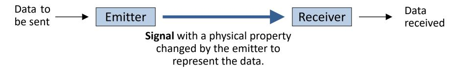
By changing signal properties like intensity, frequency or phase, data to be sent is represented, and thus transmitted along with the signal. Because they carry data, signals are also known as carriers.
