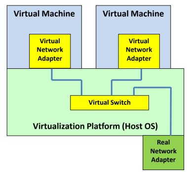
Using virtual switches connected to a real network in bridge mode is typically an option for virtual servers managed by systems administrators because it requires knowledge about the real network settings.
