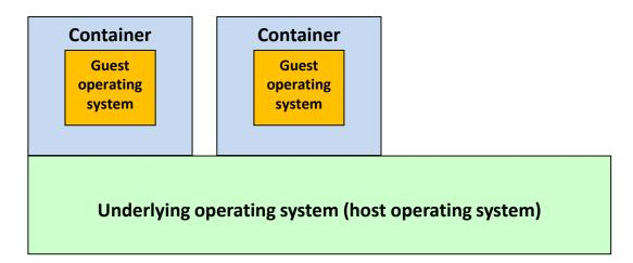
The container makes use of direct system-calls to the underling operating system, but is able to use resources only within the container.
