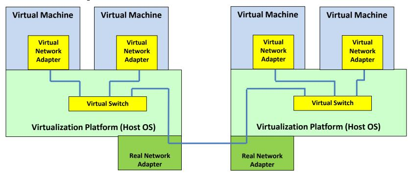
In this setup, virtual machines still aren't able to communicate with the real network, but now virtual machines hosted in different virtualization platforms are able to communicate because the two virtual switches now become a single **distributed virtual switch**.
