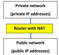
When this happens, the router stores in a NAT table the mapping between that outgoing packet and the original private address it had. Of course, later when a response to that packet arrives, it will have as destination address the router's public address. Thanks to the NAT table the router is able to match that response and will then change the destination address to be the initial source address within the private network.
