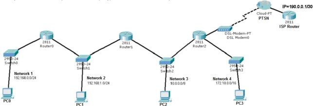
To establish the layer two connection, configure the cloud associating the DSL connection to the Ethernet connection
