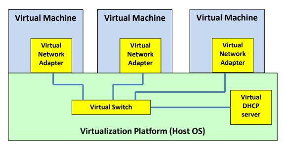
On the image the virtual switch isn't connected to any real network, so it will allow communications only between virtual machines connected to it.
