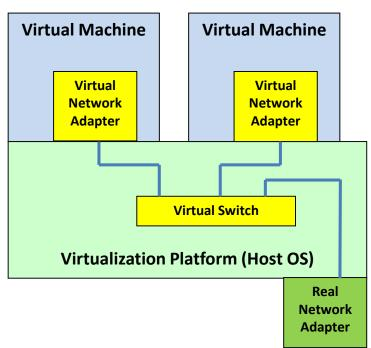
Using virtual switches connected to a real network in bridge mode is typically an option for virtual servers managed by systems administrators because it requires knowledge about the real network settings.
